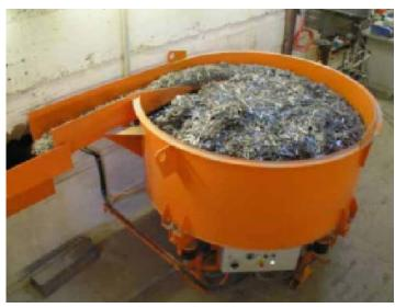
The doser's capacity goes from 150 upto 3000 L which allows a net weight of 50kg to 1200kg (100->2400 lb)
