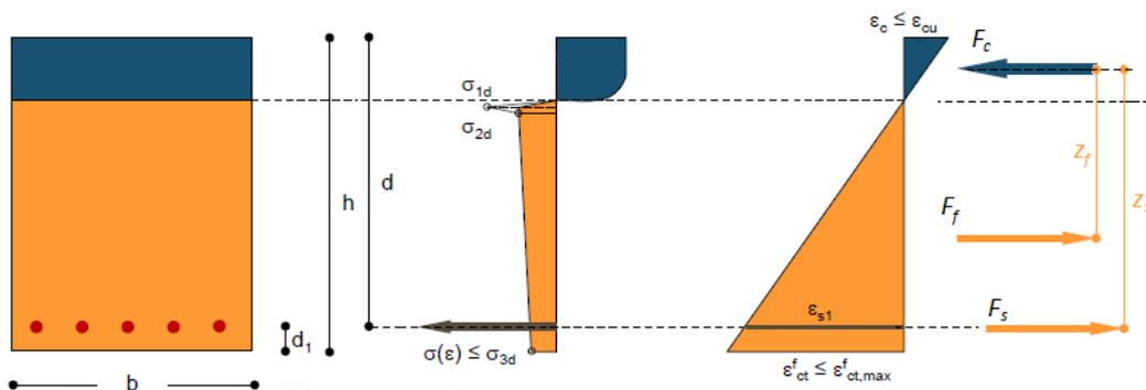
**Figure 5. Static equilibrium of the cross section under bending.**
