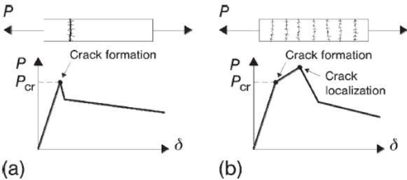
Figure 2. Typical load-deflection curve for SFRC: (a) Strain softening; and (b) strain hardening behaviour (fib Model Code (2013)).
