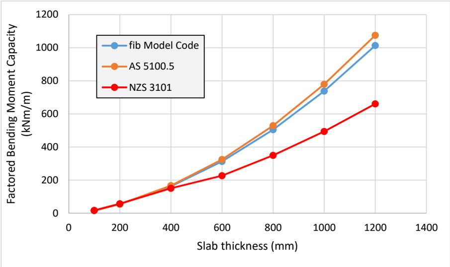
Figure 7. Ultimate bending moment capacities predicted using NZS 3101 Part 2 (2006), fib Model Code 2010 (2013) and AS 5100.5 (2017).
