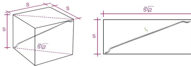
**Figure 8. Minimum dosage based on minimum overlap concept.**
