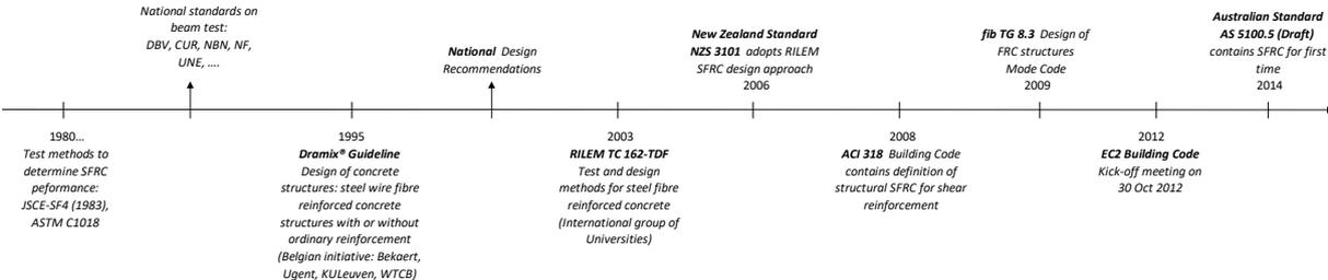
Figure 1. Evolution of SFRC test and design standards from 1980 to present.
