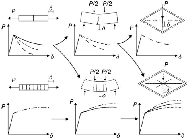
**Figure 3. Different response of structures made of SFRC having a softening or hardening behaviour under uniaxial tension or bending loads (fib Model Code 2010 (2013)).**
