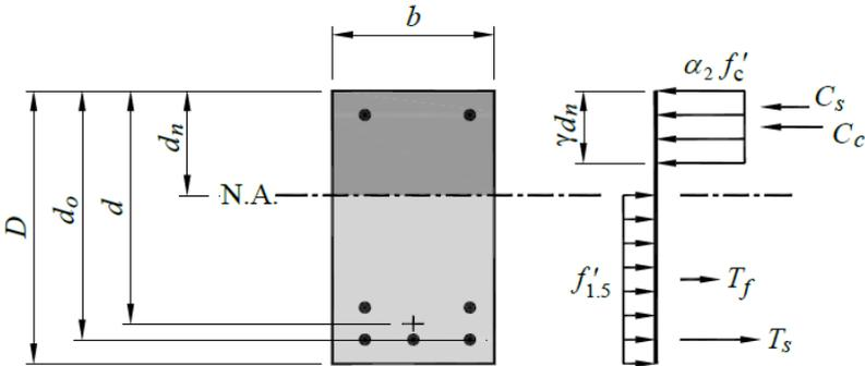
Figure 6. Design for bending in accordance with AS5100.5 (2017).
