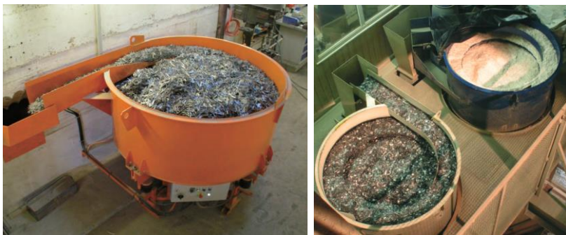
Figure 5 – Automatic fibre dosing equipment (Source: Incite AB)
