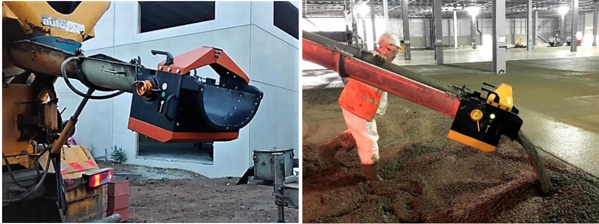
Figure 7 – Automated SFRC quality control device (Source: Bekaert)
