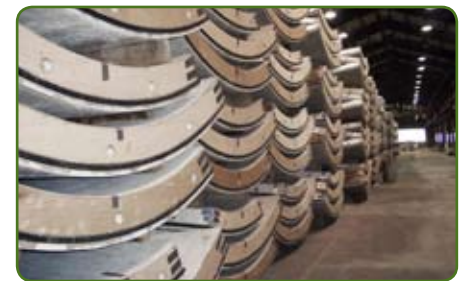
10. Steel fibres are increasingly used in arches partially or completely replacing steel armatures. Introducing polypropylene microfibres into the composition of the fibre reinforced concrete reduces the risks of scaling. The combination of steel fibres and polypropylene microfibres is therefore an optimum solution.
