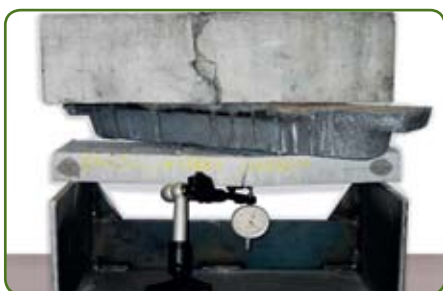
7. Creep test - only steel fibres have a creep control and as such strength on age.
