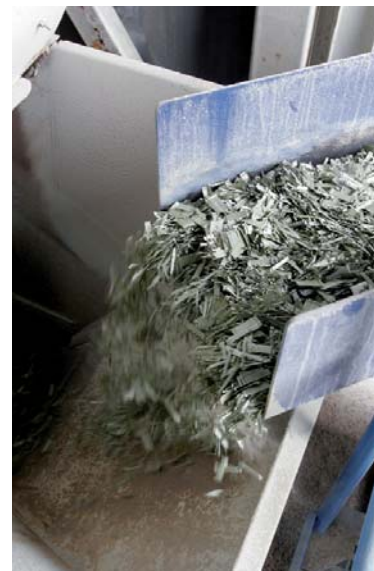
Automatic dosing of Dramix® Green into the mix.
