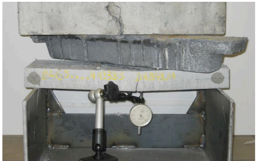
Below: Creep test - only steel fibres have a creep control and as such strength on age
