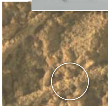
Spongy and porous surface around the galvanized steel fibres without inhibitor
