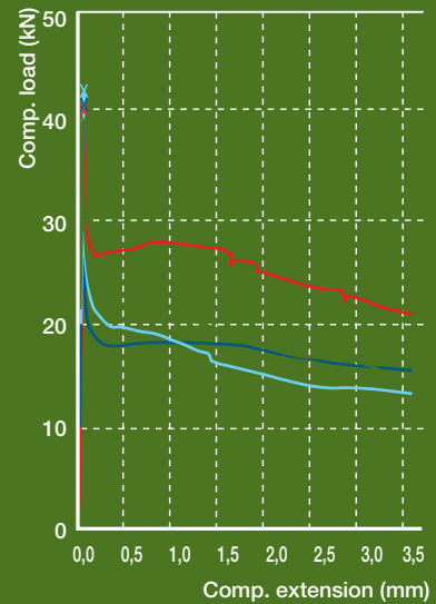
20 kg/m 3 fibres with inhibitor
